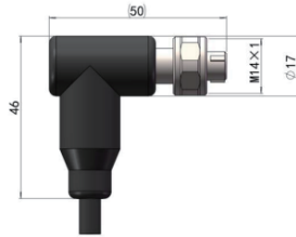
Z-MQHW14YnETK-R(P)(S)Lm Right-Angle Plug
