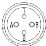
Config: 2 Fiber & 2 Contact (φ1.25) Multimode Current per Contact: 3A Insertion Loss: 1.2dB Working Voltage: ≤300V DC/AC rms Dielectric Strength: 1000V DC
